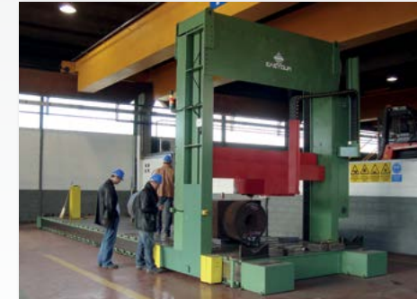
PORTALE: CNC portal for Brinell tests up to 3000kgf, 14 m, 4 axes with programmable milling included and automatic test cycle with image analysis.
